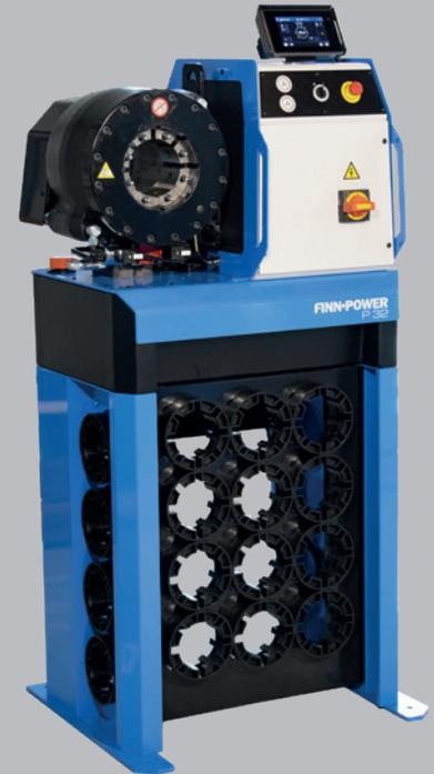
Tool rack with QuickChange-tool as an option.
